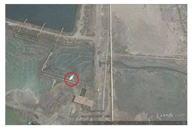
Figure 3: Google Earth image showing ash water leakage from ash water recirculation system of North Chennai Thermal Power Station into the local water body.
