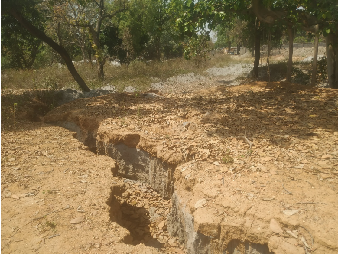
Figure 12: Ash dump near Konar Dam -Cracks in ground reveal layers of ash among layers of soil; flyash piles in the background also visible
