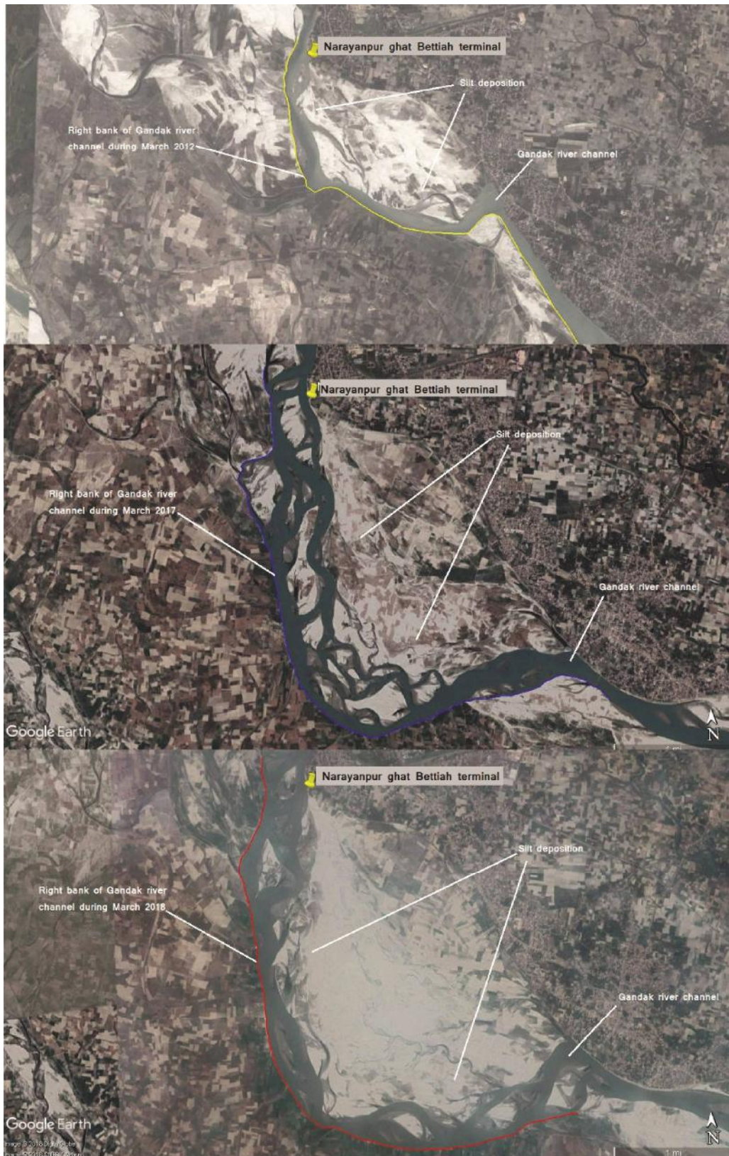
Figure 3: Maps showing shifting channels of Gandak river near proposed Bettiah terminal for NW-37. Google Earth images of Gandak river from 2012, 2017, and 2018 (top to bottom).
